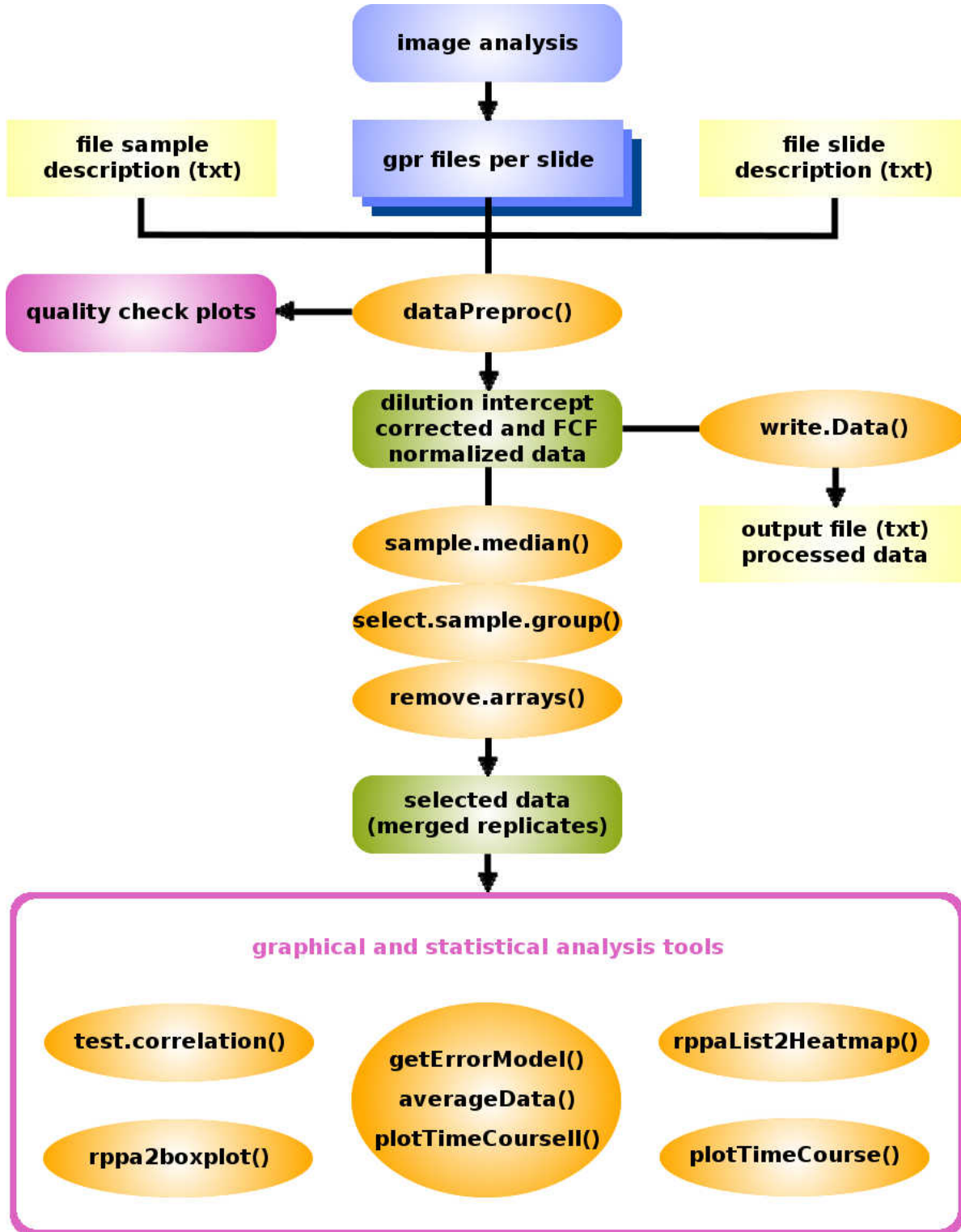
Figure 1: Recommended workflow for the analysis of reverse phase protein array data using the RPPanalyzer package
